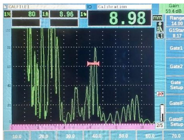
Figure 2. An example screenshot of a UT device screen during ultrasonic sound velocity measurement
